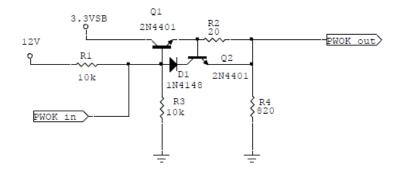
Note: The Power Ok circuits should be compatible with 5V pull up resistor (>10K) and 3.3V pull up resistor (>6.8k)
